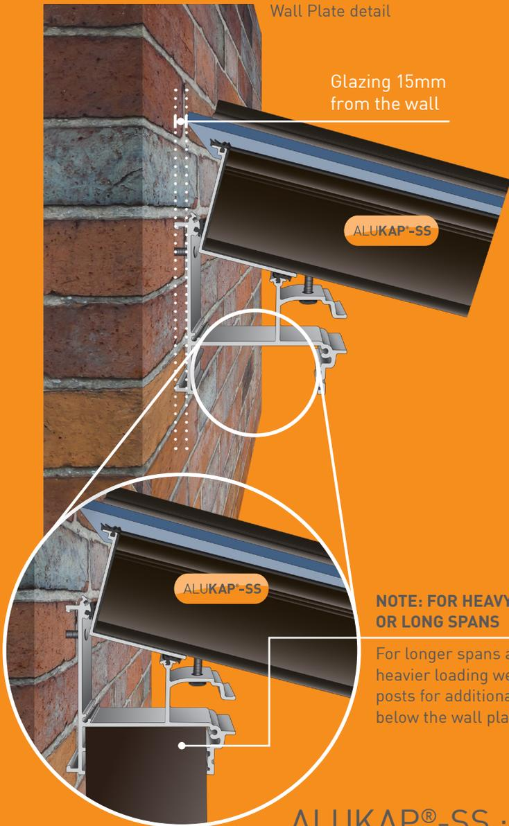
At the ALUKAP®-SS Wall Plate end, deduct 15mm from the top end of the glazing material to allow for expansion and contraction. The lead flashing from the wall should then come down and dress over this. On lower pitched roofs the flashing should be sealed on to the glazing with a compatible sealant in order to prevent water ingress in severe weather.
